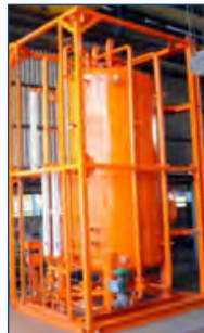
SURGE / GAUGE TANK
